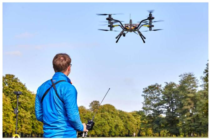
Drone geophysics can be used to reliably detect pipelines and explosive ordnance
