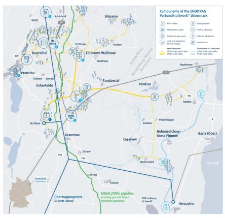
The ENERTRAG Integrated Power Plant® Uckermark at a glance: Already a reality, the Uckermark plant generates clean electricity, green hydrogen, and heat over an area of  $40 \times 40$  kilometres.
