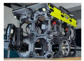
ROV in Light-Work-Class-Configuration with manipulator and additional payload-level
