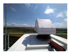
Gondola-mounted lidar on the wind turbine OPUS 1
