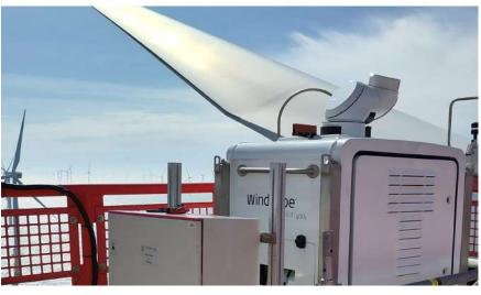
Scanning Lidar device on the nacelle of a wind turbine at RWE's offshore wind farm Amrumbank West. © Jörge Schneemann [2024]
