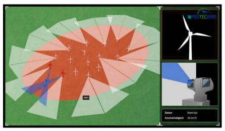
AVES wind anti-collision system: Schematic representation of the triangulation of a red kite with two wind turbines
